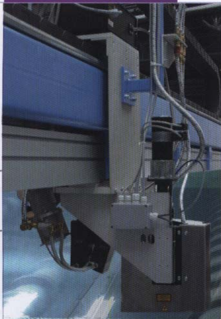
TMF cold-end system with strain measurement
