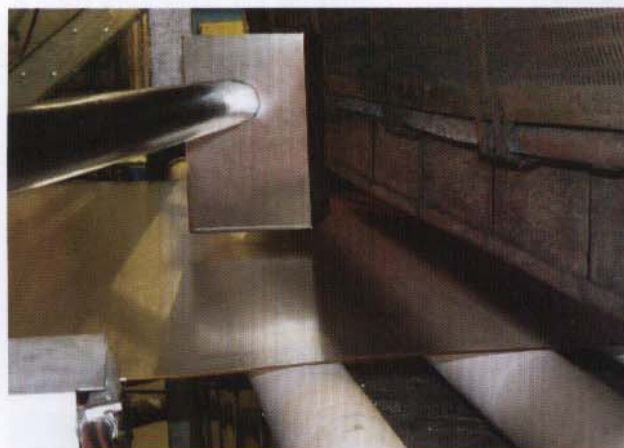
Patterned (solar) glass thickness measurement system for hot end applications.
