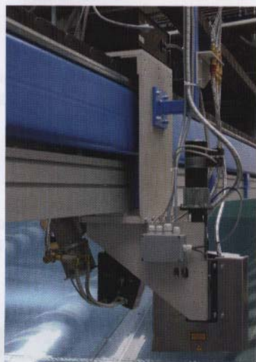
Overview of VMA's TMF system for float glass thickness and strain measurement.
