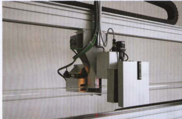
Off-line tube inspection system.
